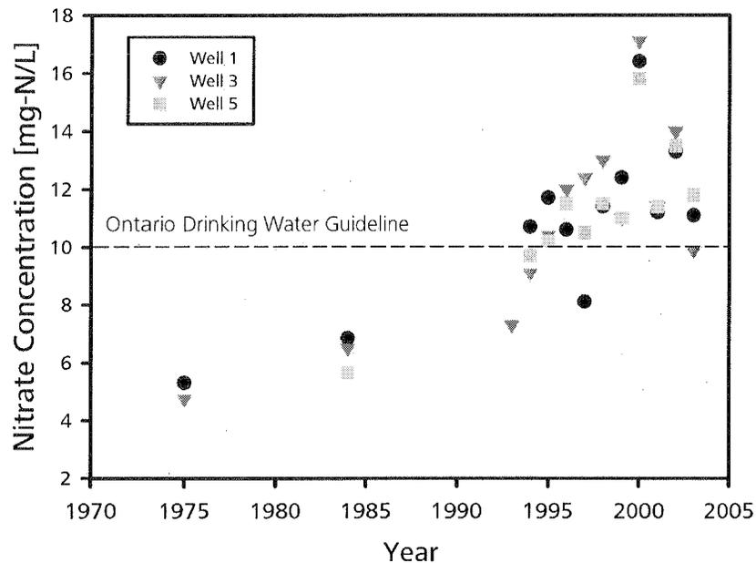
**Fig. 3** Maximum annual nitrate concentrations (mg N l<sup>-1</sup>) observed at three of the five extraction wells in the Thornton Well Field.
