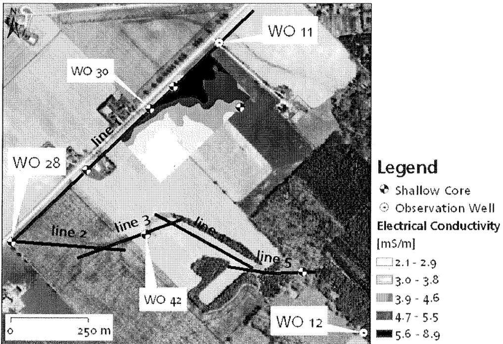
Fig. 5 Location of the five resistivity survey lines, and the area covered by the EM survey.
