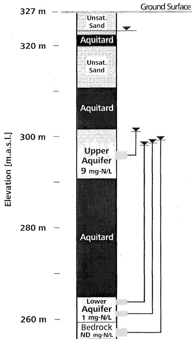
Fig. 4 Stratigraphic log of borehole WO 28 showing the location of the screened intervals, the associated water level for each observation well, and the nitrate concentration measured in each water bearing zone.
