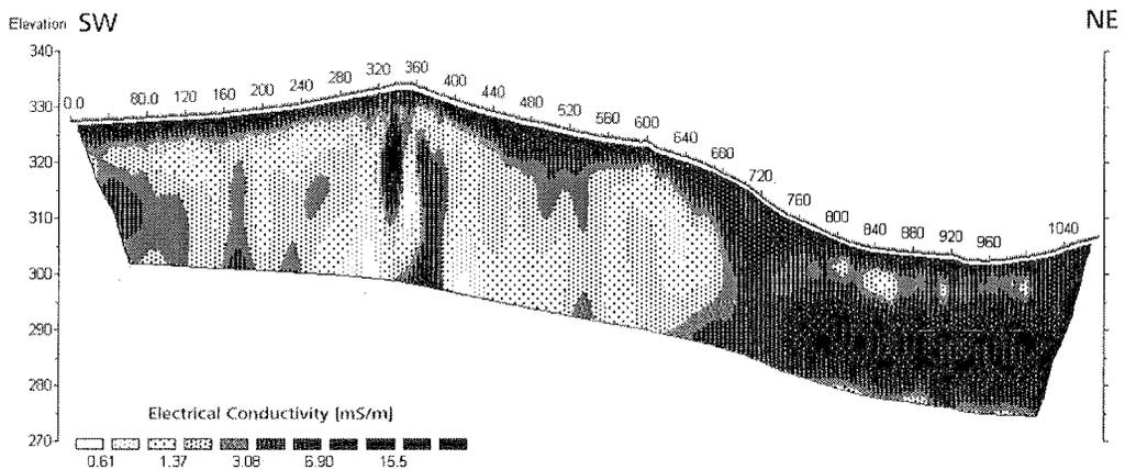
Fig. 6 Results of the Resistivity survey along Line 1.
