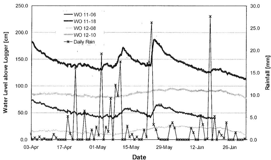
Fig. 7 Water level response at two discrete depths in wells WO 11 and WO 12 (see Fig. 5 for locations). Monitoring piezometers WO 11-06, and WO 12-08 are the shallow piezometers at each location.
