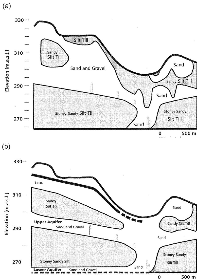
**Fig. 2** Cross section of the conceptual hydrostratigraphic model through the five supply wells of the Thornton Well Field (indicated as screened intervals): (a) initial conceptual model after Padusenko (2001); and (b) revised conceptual model as a result of the findings discussed in this paper.
