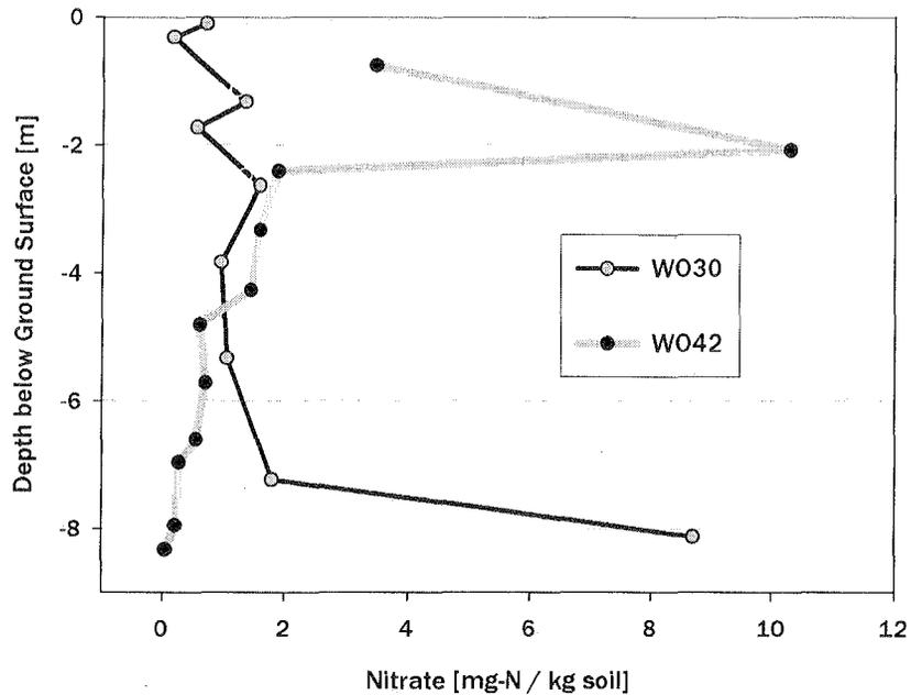
Fig. 8 Example bulk soil nitrate concentration profiles. Core WO30 was extracted from a location where sand overlies the shallow aquitard which was present at a depth of 8 m, and Core WO42 was extracted from a location where the upper 8m consists of silty till material. Core locations shown on Fig. 5.
